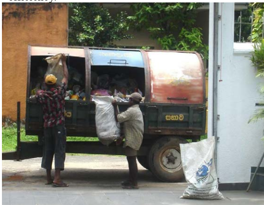
Tractor-trailers are suitable for transport over short distances. They are also suitable for the collection of recyclables as waste can be loaded separately by type.
