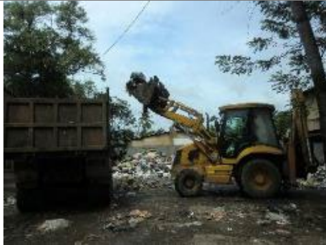
Gampaha MC Waste transfer is entrusted to a private company. Waste is transferred three times a day by 20 m 3 dump trucks.
