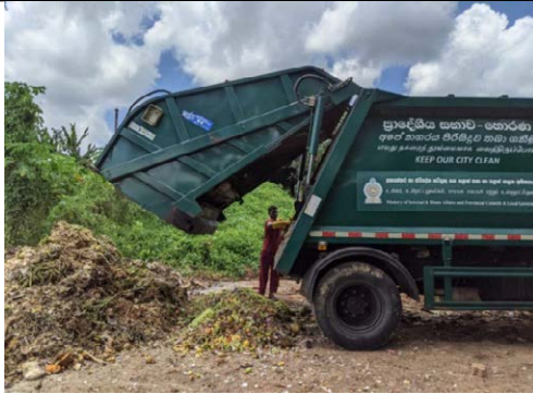
Compactor trucks are suitable as collection vehicles for organic and other waste due to their high collection efficiency.
