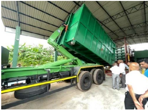
Container hauler trailer vehicle with hook system
