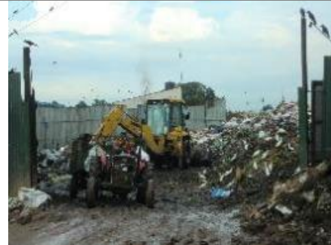
Kolonnawa UC Collected waste is generally unloaded separately into two piles (biodegradable and other waste) at the transfer station. Collection vehicles, transfer equipment and vehicles operate in a very narrow transfer space.
