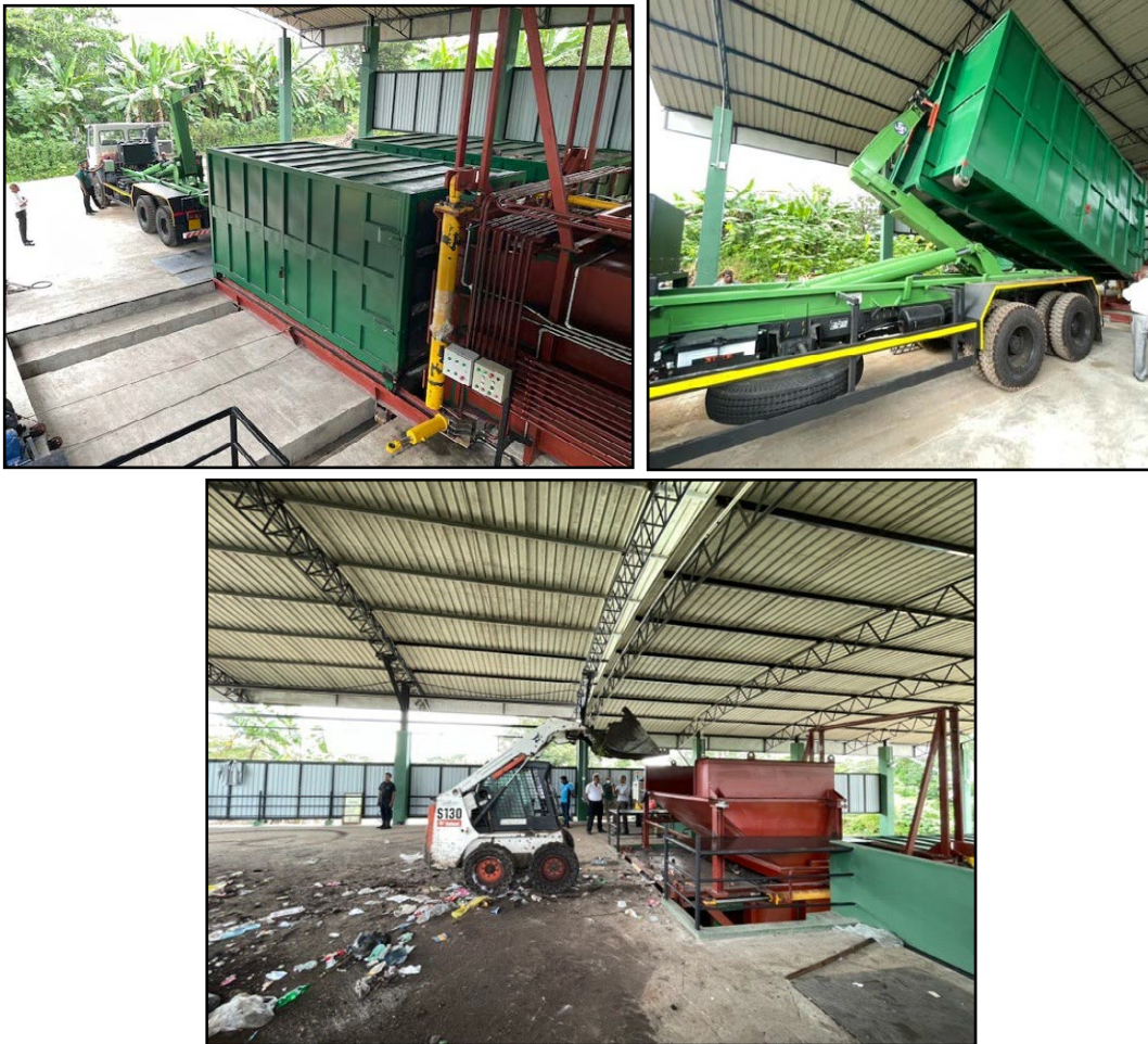
Figure 6 Equipment to be used at the Transfer Station (Waste container+ Container hauler vehicle with hook system + static compactor with input hopper)
