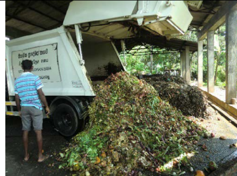
Compactor trucks are suitable for the collection of biodegradable waste as they can prevent wastewater leaks and offensive odors.
