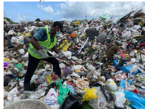
Moratuwa MC Non recyclables such as polythene sorted from non-biodegradable waste are baled and transported to a cement factory, INSEE, as fuel substitute.
