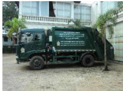
Gampaha MC Compactor truck with 6-ton loading capacity donated by MoPAHAPCLG
