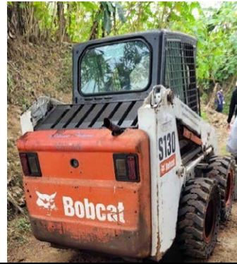
Bobcat used to feed hopped with waste
