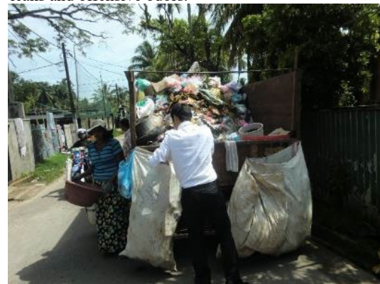
Tractor-trailers are suitable for transport over short distances. They are also suitable for the collection of recyclables as waste can be loaded separately by type.
