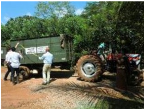
Horana PS This type of tractor-trailer with a loading capacity of 6.6 m 3 is a typical collection vehicle in the Western Province
