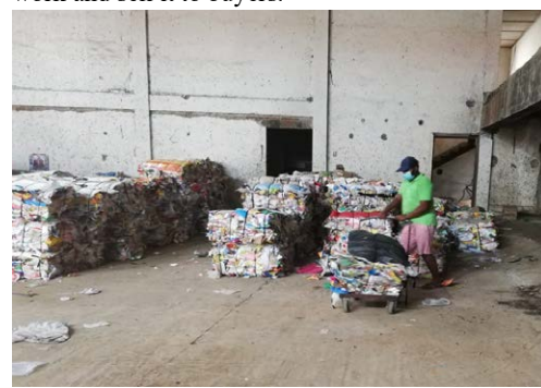
Moratuwa MC Non recyclables such as polythene sorted from non-biodegradable waste are baled and transported to a cement factory, INSEE, as fuel substitute.
