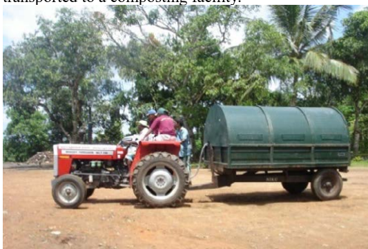
Bandaragama PS Half cylindrical collection trailer with slide-type lid (6 m 3 ).
