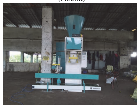
袋詰め機械 (Compost bagging Machine)
