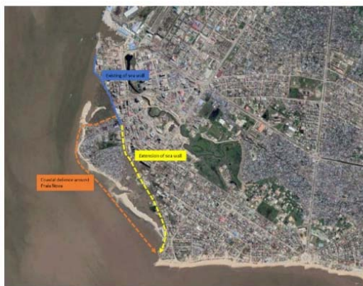
Figure C.24: Two routes for protecting the city of Beira against hazards from sea.
