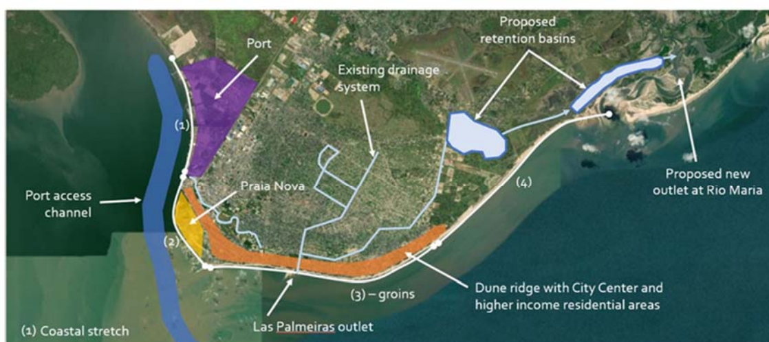
Figure 2-1: Beira project area with 4 distinguished coastal stretches
