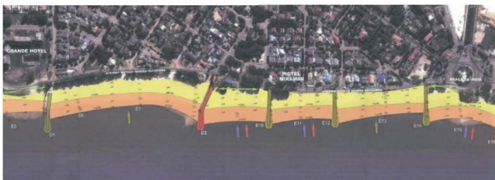
Figure C.23: Redesigned coastal protection scheme with higher and wider dune area and reinforced groyne (Source: [Consulmar, 2012])
