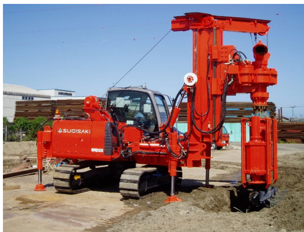
Figure 7.4.40 Photograph of Installation Equipment of Diaphragm Wall under Limited Clearance
