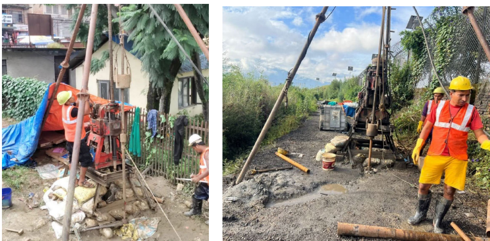
Photo 3.3-2 Ongoing SPT assembly at drilled hole BH3 and BH4
