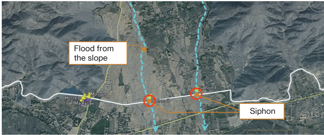
Figure 4.50 Siphon Installation in the Flood Area 2)
