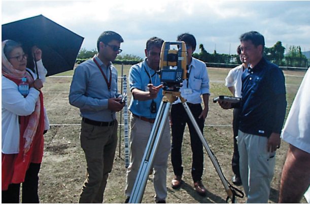
Auto Tracking Type of Total Station 2)
