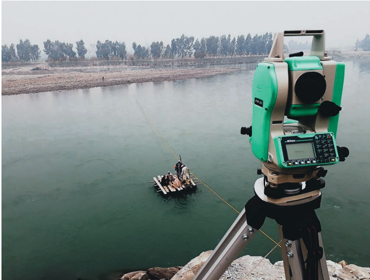
Photo 3.7 River Survey by Total Station 2)
