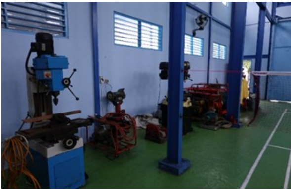
Drilling machine and grinder
