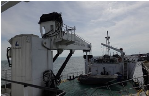
Main and auxiliary crane
