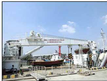
Crane system (New Buoy Tender)
