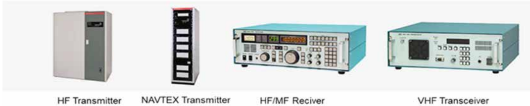
Picture 7.2.3 -1 : GMDSS Equipment in Operation
