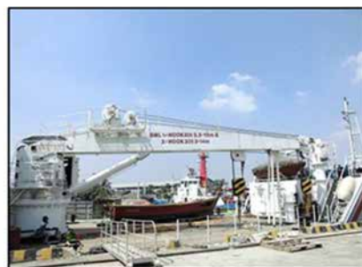
Crane system (New Buoy Tender)
