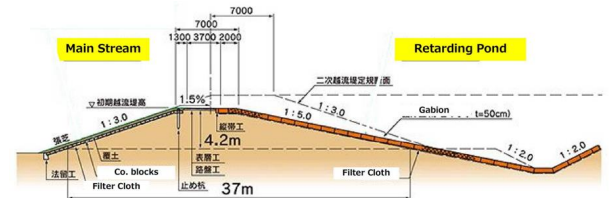
Figure 5. Example section of overflow dike.
