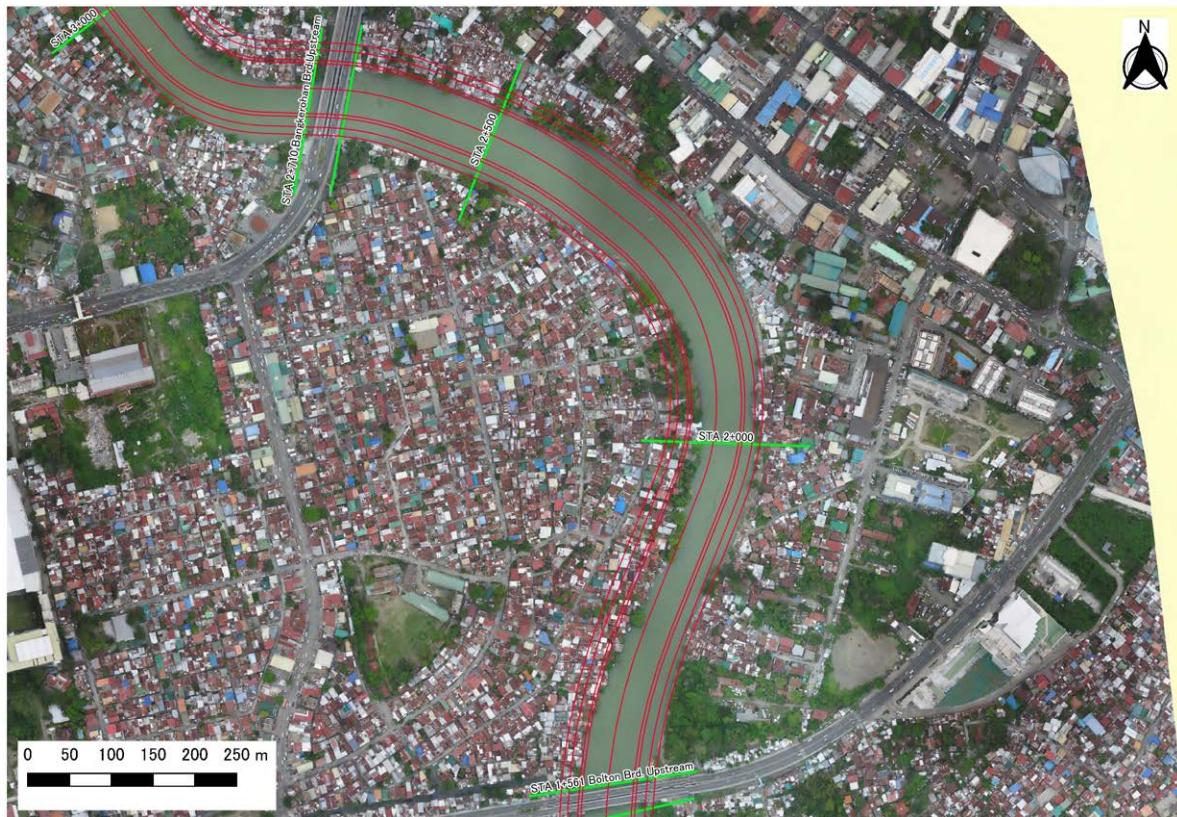
Figure 5.1.9 Design Alignment of Alternatives of River Widening (Alt.1)
