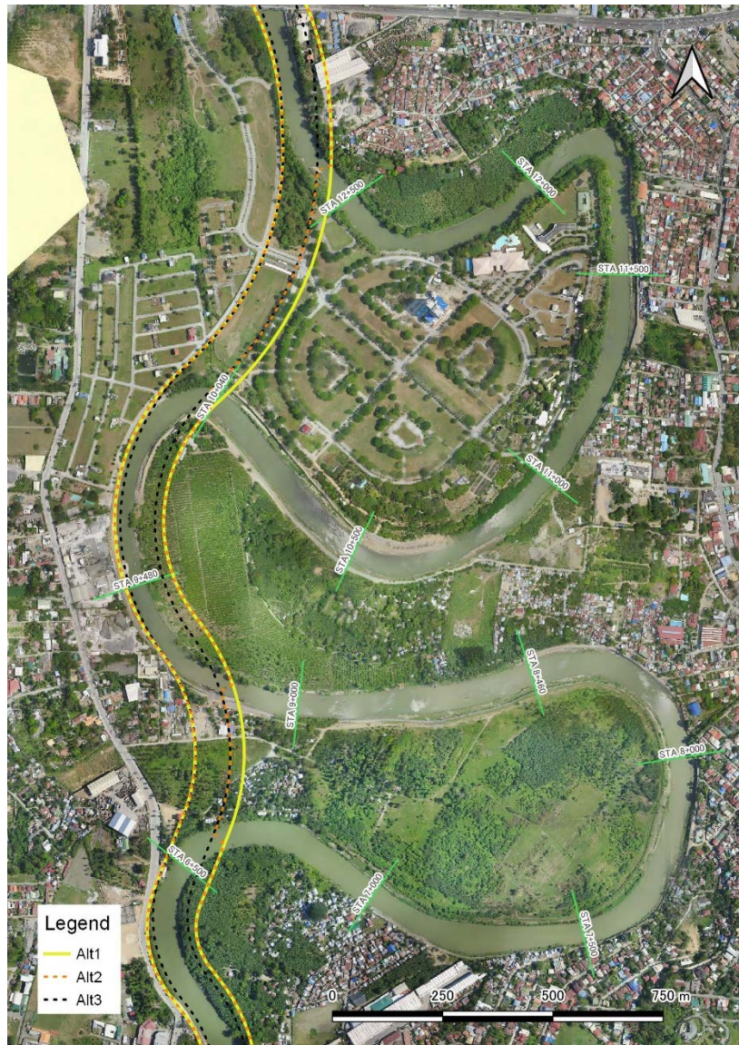
Figure 4.1.15 Design Alignments of Cut-off Portion
