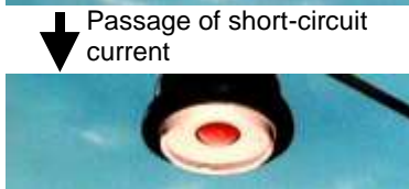
Indication changes of OC (by electricity)
