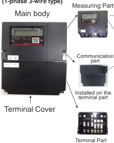
[Structure (Image) of a smart meter] (1-phase 3-wire type)
