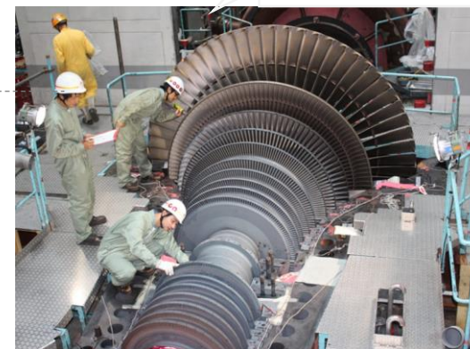
Conventional Generator (Rotary synchronous generator)
