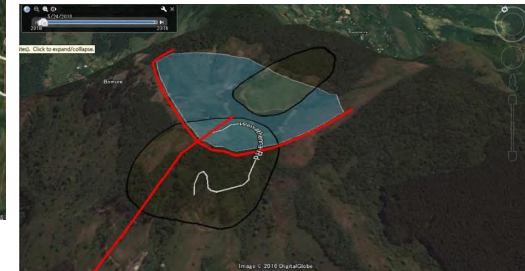
Upper reservoir and Possible landslide (black line)
