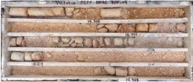
Fragile core sample (BH-02: 15-20m)
