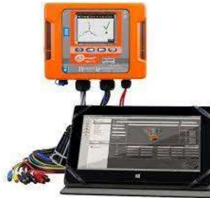
LECO Procured Power Quality Analyzers
