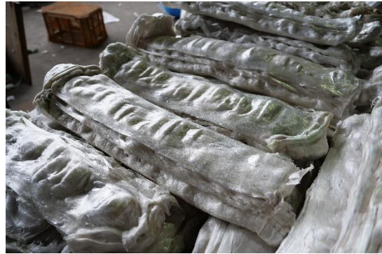
Photo 6-47 Volume Reduced Styrofoam
