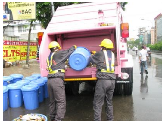
Photo 33 Waste Collection by Compactor (Fixed-Place Collection at Regular Intervals)
