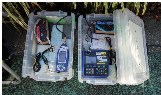
Photo 1-12 Installed Sound Level Meter and Vibrometer
