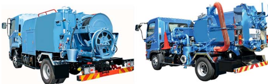
Figure 1-14 High-pressure Drainage Cleaning Vehicle (Left) and Sludge Suction Truck (Right)
