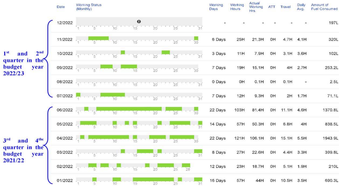
Source: Collected data from the GPS tracking system of excavator (PC220-8M0, 100865)
