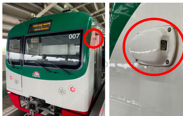
Source: JICA Expert Team CCTV Camera
