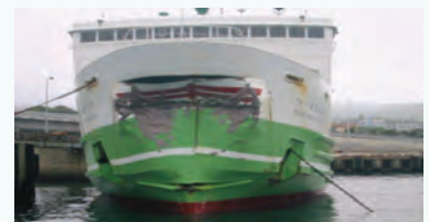
Ferry breakwater collision (23 injured)
