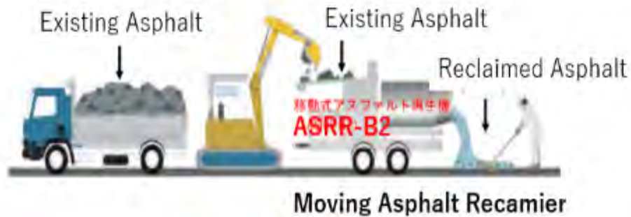
Fig. 2 Pavement Rehabilitation Method Using ASRR-B2
