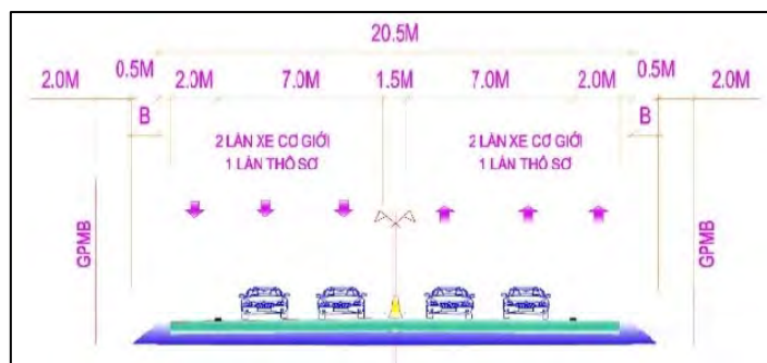
Figure 6.1.6 Proposed Cross-section in the Current Project Proposal
