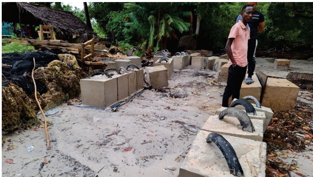
Fabricated 36 pcs. concrete mooring blocks in Kijiweni
