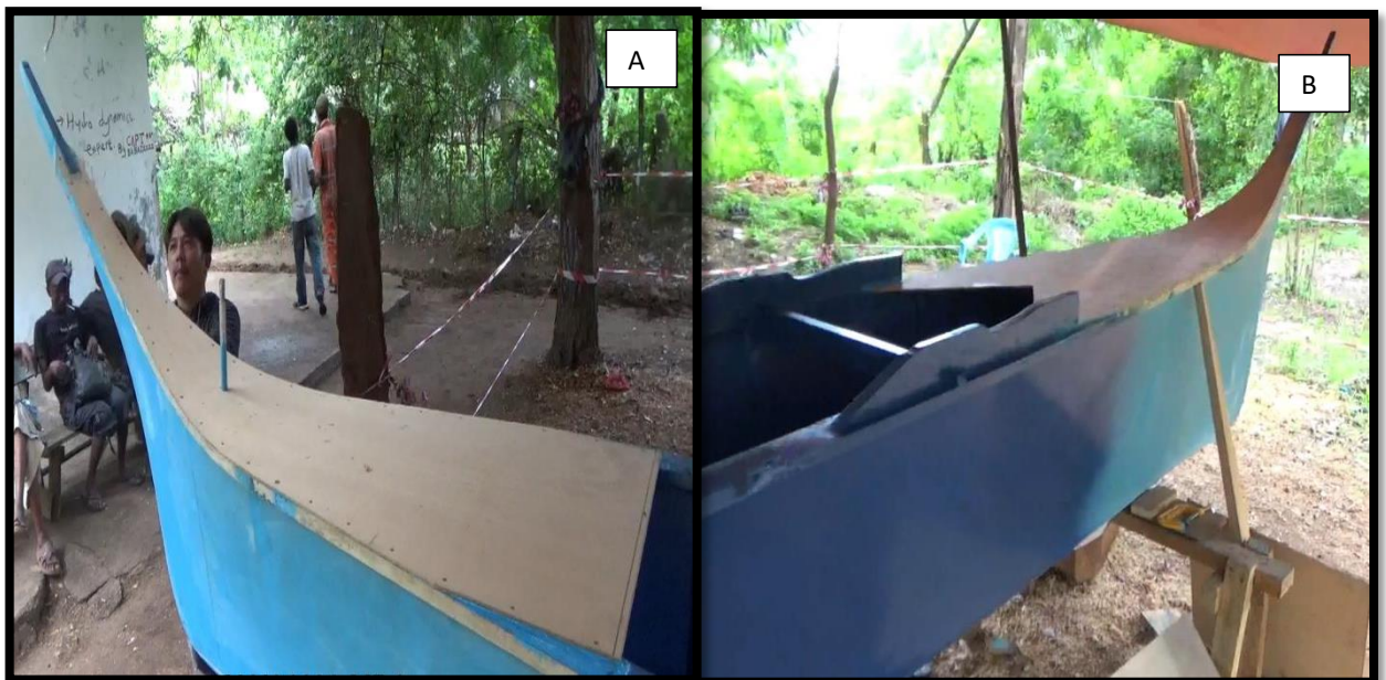
Figure 20. Planking of plywood on (A) bow and (B) stern deck of the boat.
