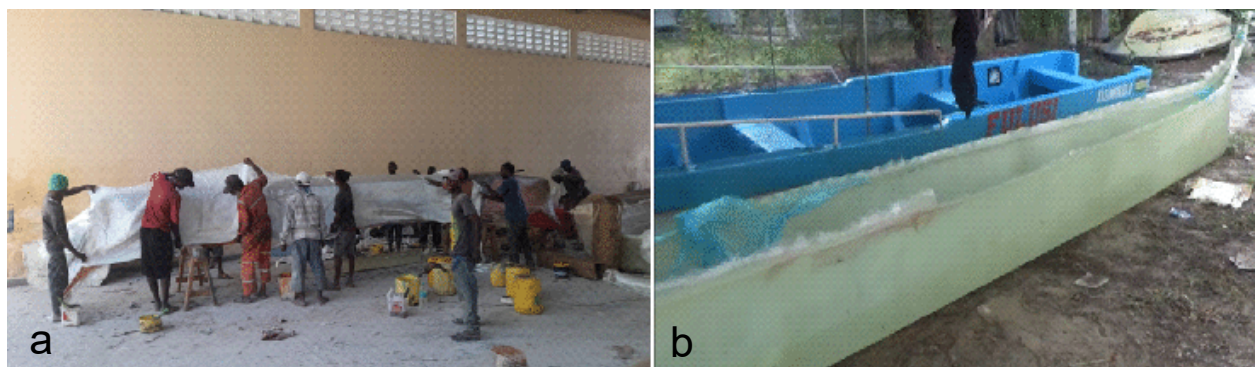
Figure 45. FRP fabric being stretched over a wooden banca boat to make a FRP mold (a); FRP banca hull taken out (b).
