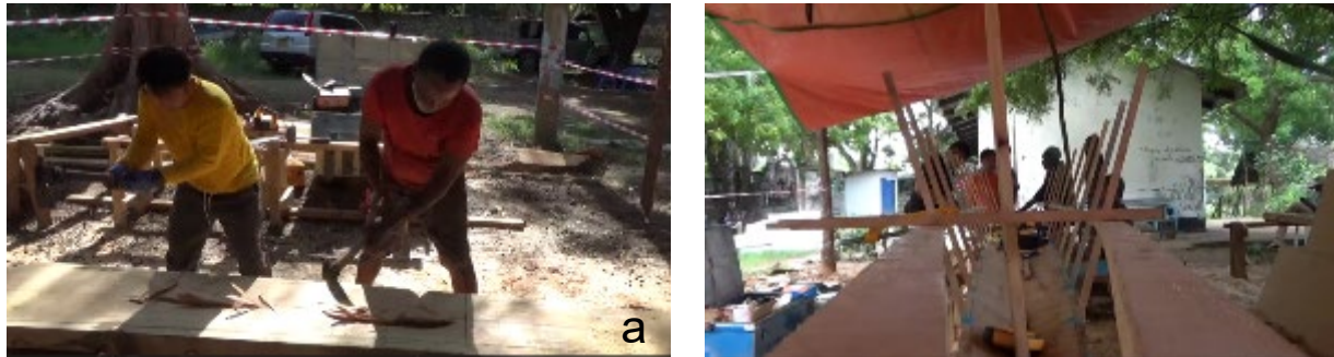
Figure 41. Boat Building Works: Keel being hollowed out by hatchet (a), Ribs being assembled (b).
