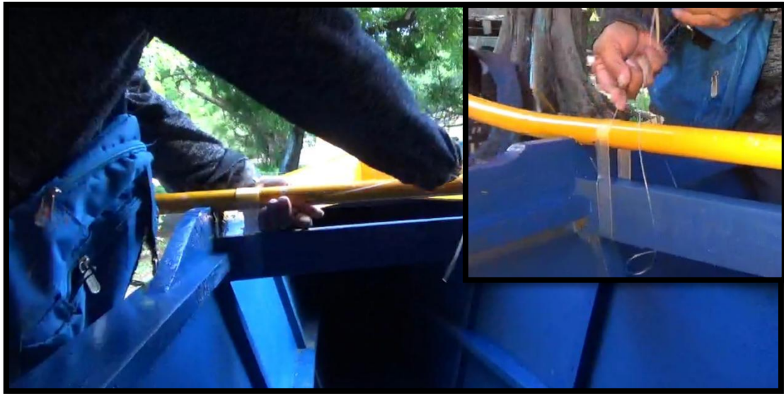
Figure 26. Tie lashing the outrigger boom to the brace below the outrigger boom stand with the use of monofilament nylon.
