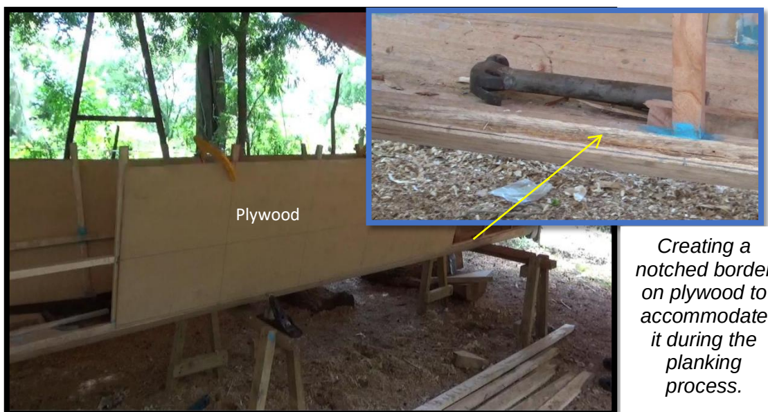
Figure 14. Measuring and planking of plywood to the boat frame.
