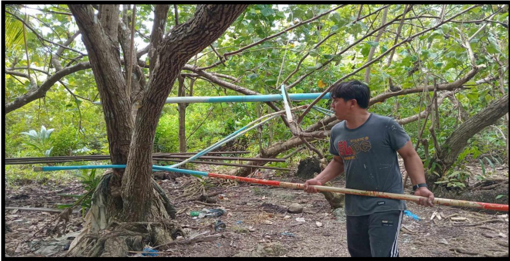
Figure 25. Bending of outrigger beam using GI pipe material.
