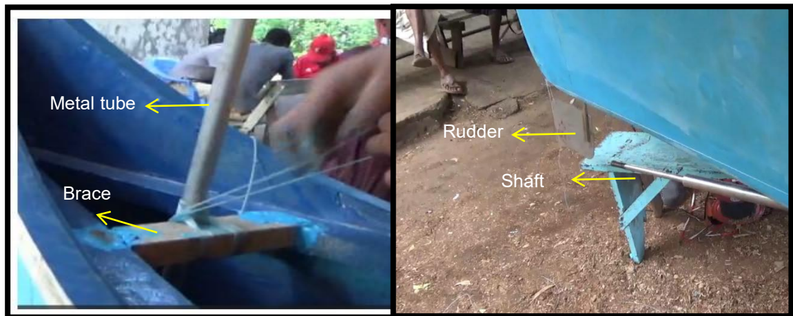
Figure 34. Secure the metal tube to the brace with nylon, then attach the rudder to complete the assembly.
