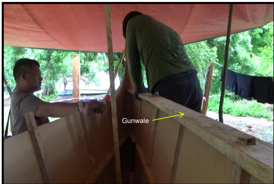
Figure 15. Photo showing the part of the gunwale. Excess ribs should be cut to attach the gunwale on top of the frame.
