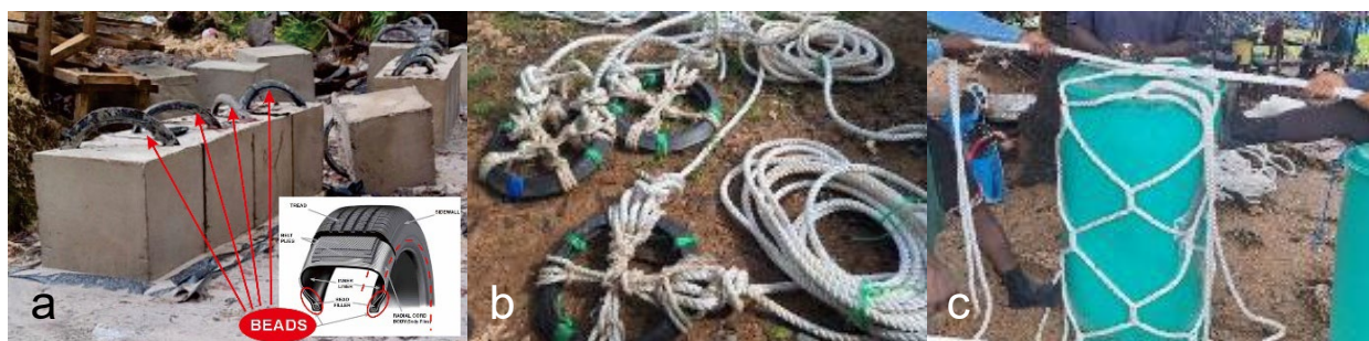
Figure 53. Concrete anchor block using tire beads for rope attachment handle (a), grid mooring rope frame using tire beads for rope connection ring (b), large 200L float using used PE drum (c)
