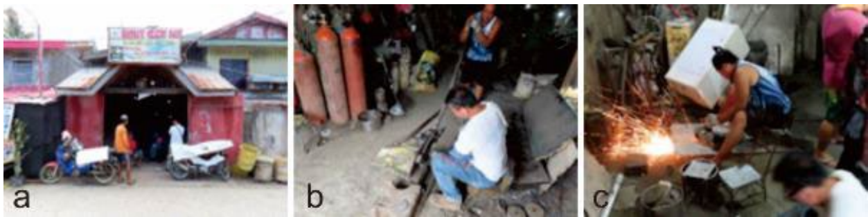
Figure 47. Specialist cottage industry shop in stainless steel fabrication of propellers, rudders, etc. for Banca boats in the Philippines (Catbalogan, Samar Province)
