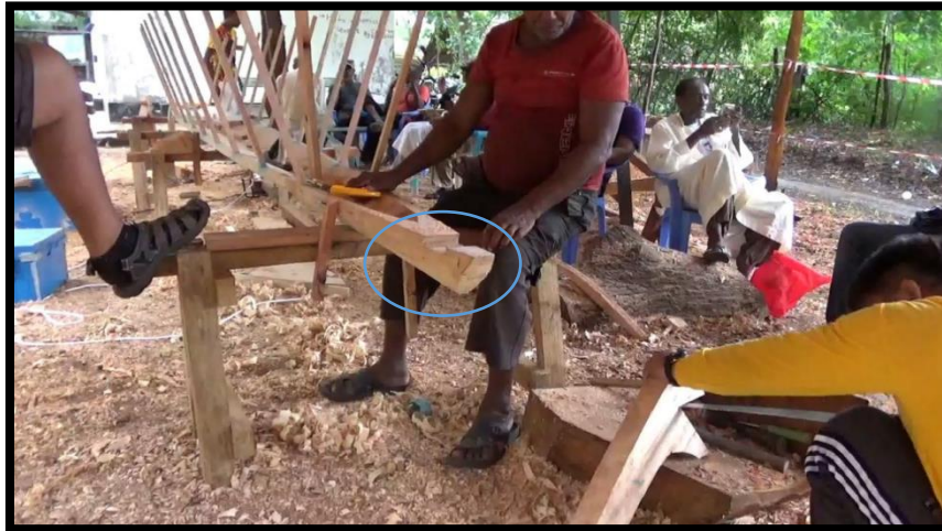
Figure 9. Carve out space for the attachment points of both the bow and stern.
