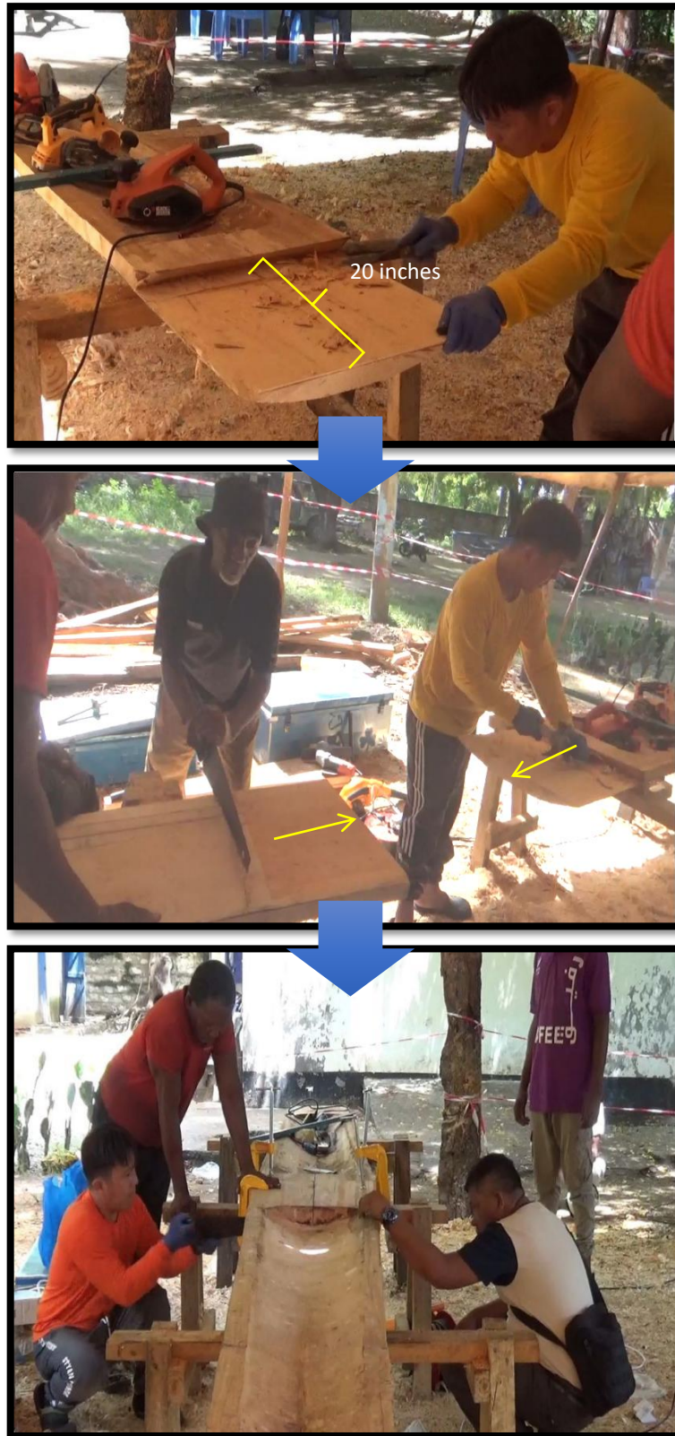
Figure 6. Measuring and carving the keel to align with the extended keel.
