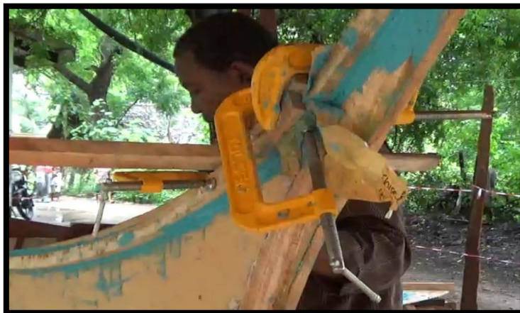
Figure 17. Use epoxy to adhere the gunwale along the upward curbed bow-end part of the boat and secure it in place with a G-clamp for support.
