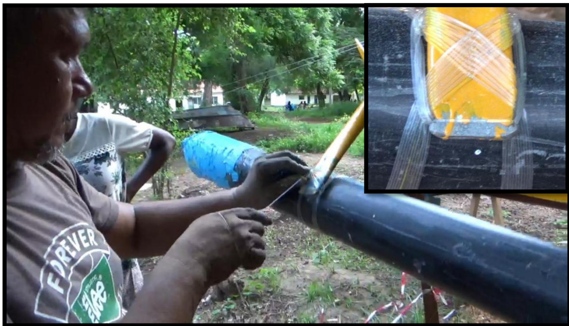
Figure 27. Lashing the outrigger boom to the outrigger boom stand using monofilament nylon.
