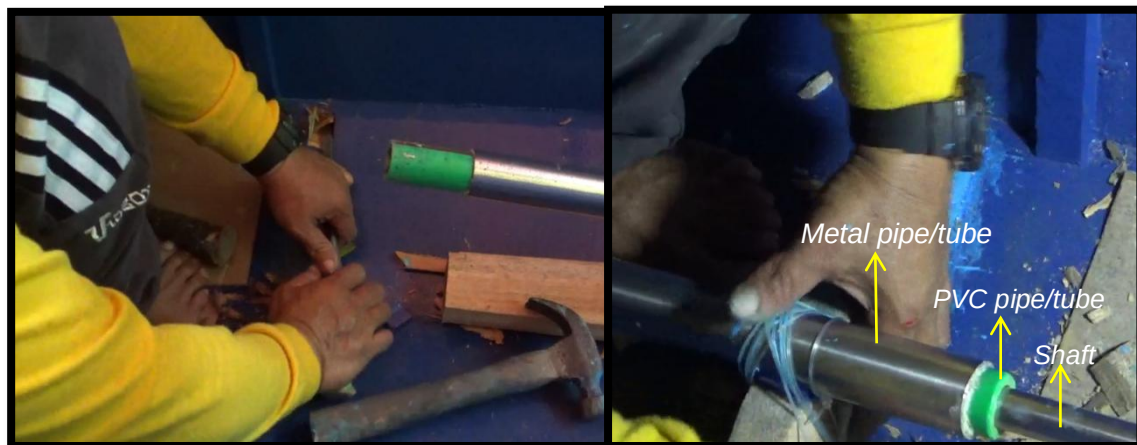
Figure 30. Creating a support or breaker for the propeller shaft to minimize the vibration of shaft when operating the engine.
