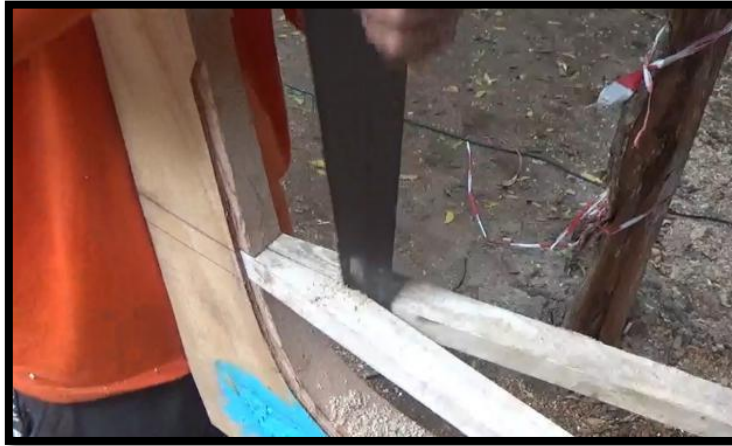
Figure 13. Joined the ends of the two gunwales and secured them to the stern.
