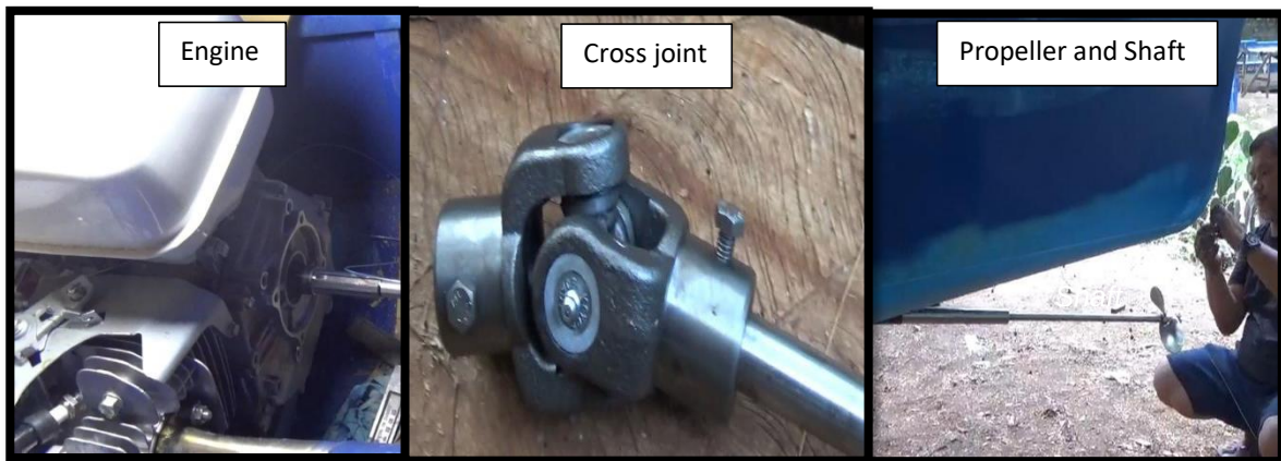
Figure 31. Insert the shaft into the metal tube, attach the cross joint to both the shaft and the engine, and finally, assemble the propeller.
