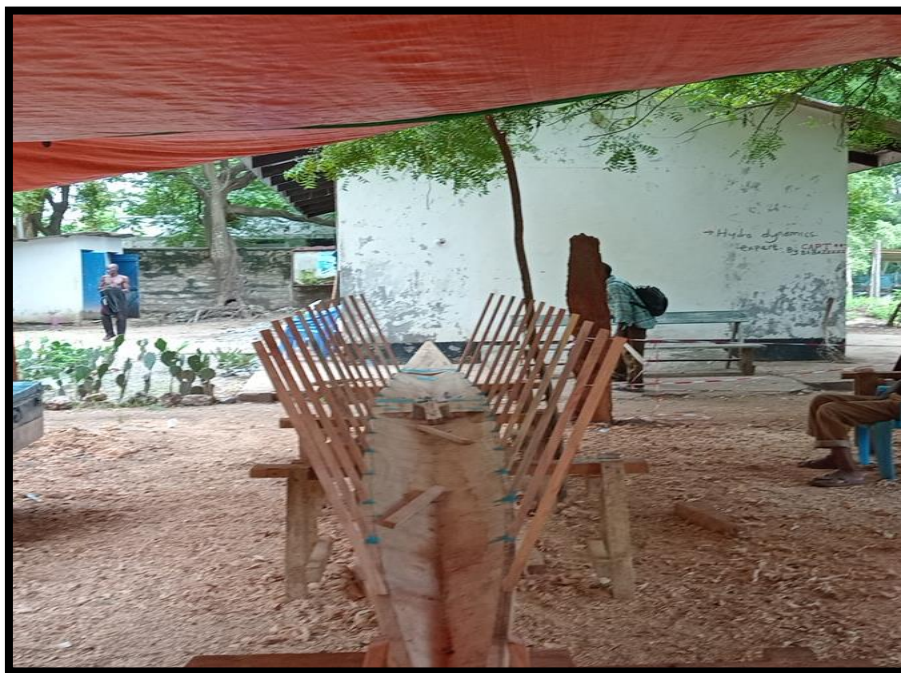
Figure 8. Attaching ribs onto the slots on the keel using epoxy
