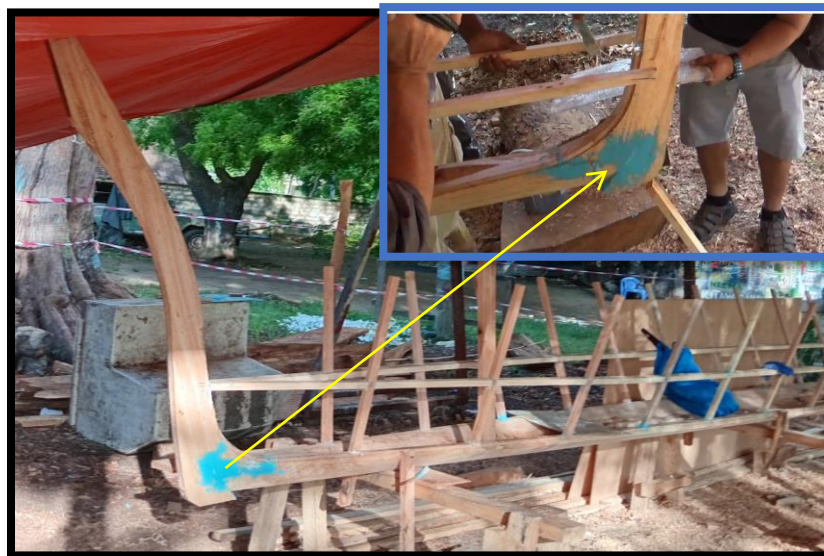
Figure 10. Attaching the stern of the boat with a 2-inch x 10-inch x 4.8 feet piece using epoxy.
