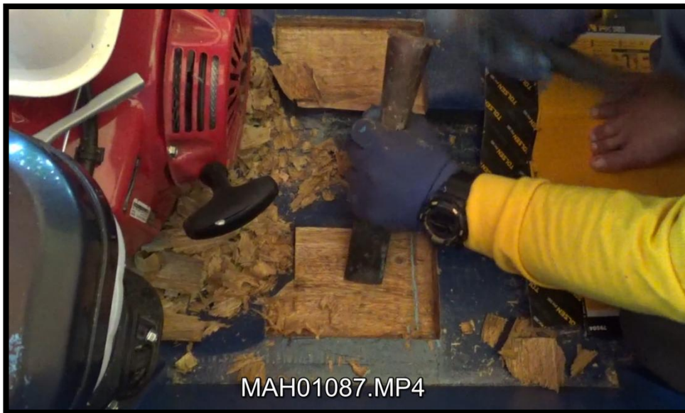
Figure 28. Creating an engine bed from a hardwood with a dimension 15 in x 8 in x 2 in.
