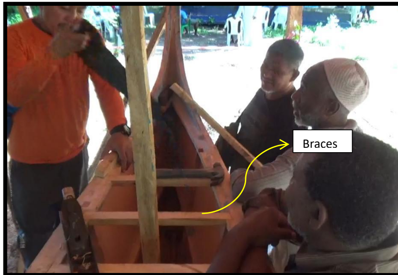
Figure 18. This photo showed the braces attached in the inward part of the stern. This serves as the support system of the boat.
