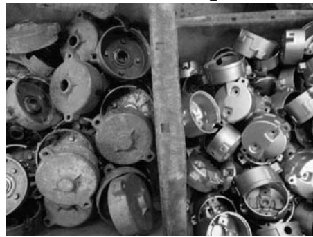
Mechanical cleaning (Shot-blasting)
