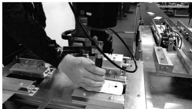
Automation of smartphone disassembly ProAutomation GmbH, Austria The development was supported by EU funded project.
