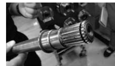
Drive shaft (Driveshaft splines restored by welding)
