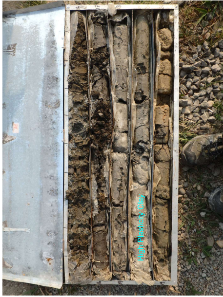
Photo-5 Core samples from borehole BGT-5 at depths of 15-20 m Highly plastic clays are recognized at depths of 17-19m.
