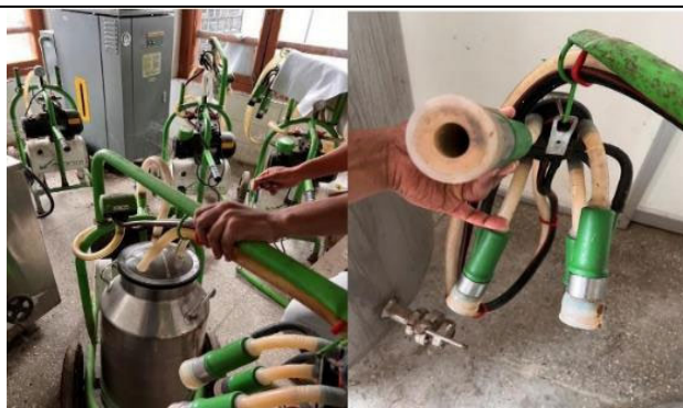
Figure 4-21 Portable milking machine and silicone liners
