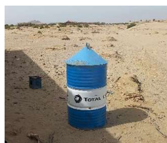
Fig 6-47 Full-size drum smoking kiln
