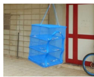
Fig 6-44 Hanging net-type dryer
