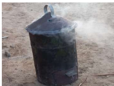
Fig 6-45 A model smoking kiln using small drums
