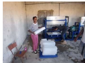
Fig 6-62 Trial run of the ice making machine, 30 ice blocks made at one batch.
