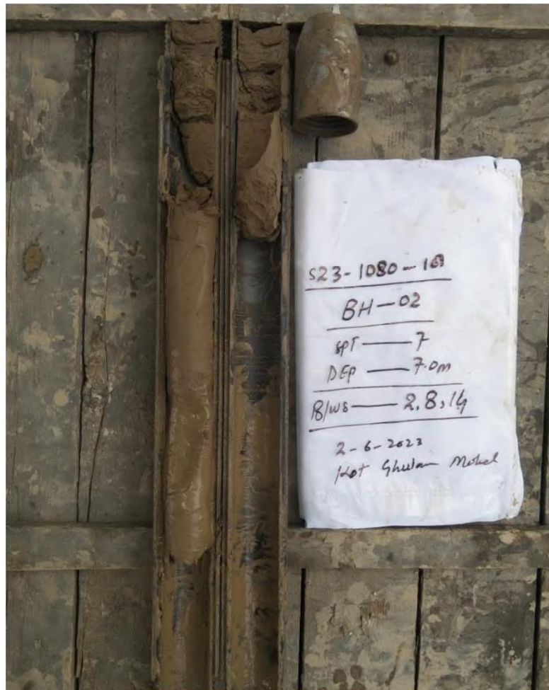
Figure A.4: Sampling via split spoon sampler
