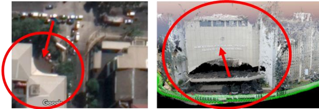
Figure II.17 Left: Ortho-photo (from Google), Right: 3D data
