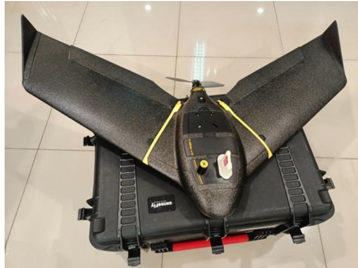
Figure II.28 Fixed-wing UAV Provided by JICA Project Team
