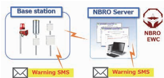
Figure 39: Structure of Warning SMS sent from Base Station and NBRO Server
