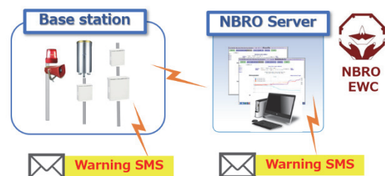
Figure 38: Structure of Warning SMS sent from Base Station and NBRO Server
