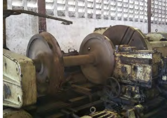
Figure 4-42 Wheel Lathe Machining at Limete Wheel Axle Workshop
