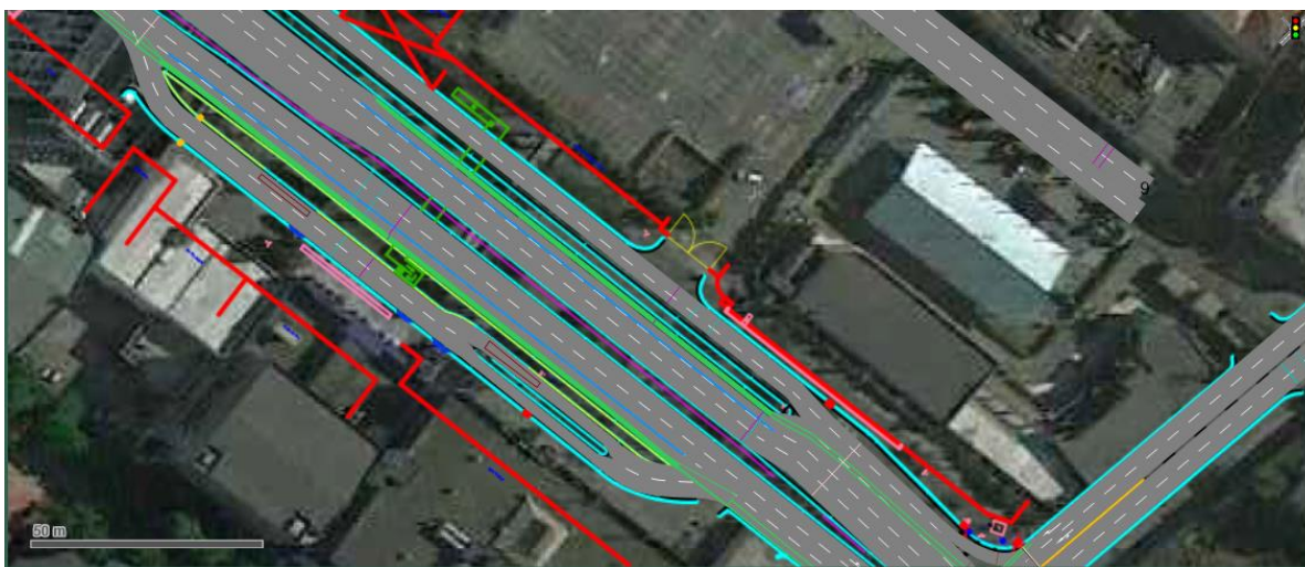
Figure 3.1: Screenshot of Simulation Model with Bicycle Lanes along the Main Road
