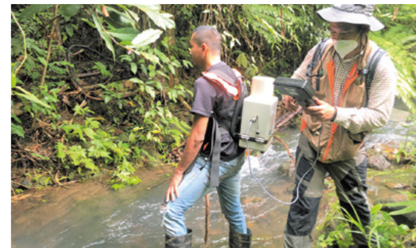
Philippines: KIZUNA participants conducting geophysical prospecting with the VLF method in a field in the province of Camarines Norte on Luzon Island
