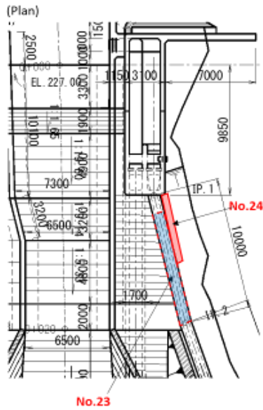
Figure 2-2-19 Rehabilitation Plan from No.23 to No.24
