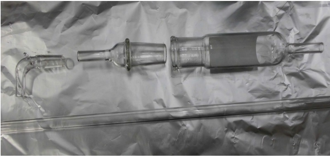
4) Nozzle, filter paper holder, and collection tube after dust recovery
