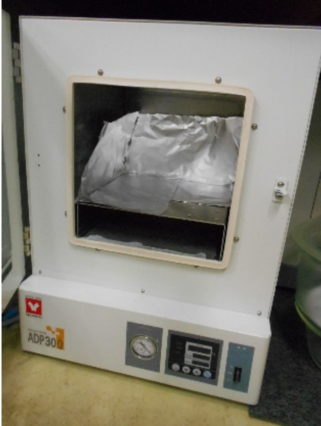
4) Vacuum dryer: used for drying XAD resins and PUF after washing.
