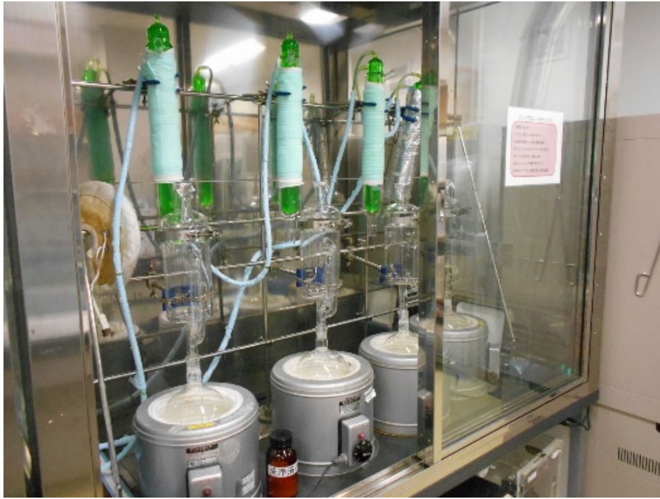
2) Soxhlet extractor for washing XAD resin (2L size)
