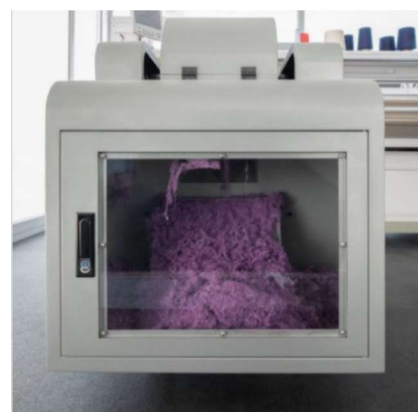
Loop machine shredding fabric
