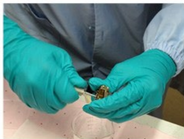
Ion source cleaning
