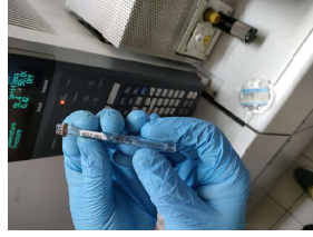
Replacing inlet liner
