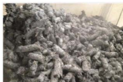
Pellets as final product from the URENCO waste treatment plant
