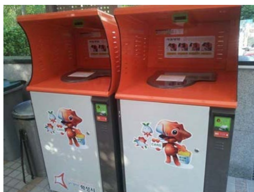
Automated bins equipped with scales and RFID Consumer uses tap card to activate automated bins
