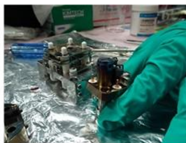
Ion source disassembly
