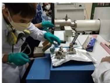
Ion source removal/ installation
