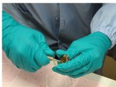
Ion source cleaning
