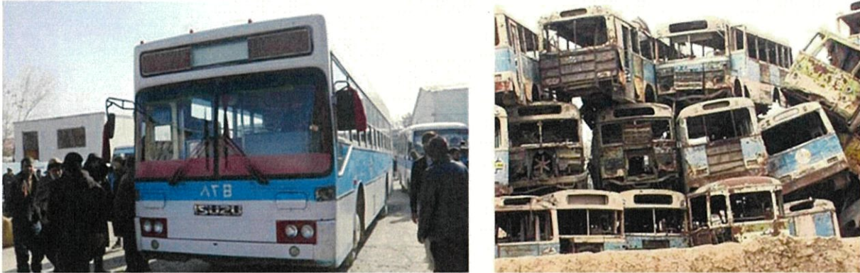
Figure 1-2-2 A. Functional Buses Donated by JICA B. Scrapped Buses Due to Lack of Proper Maintenance
