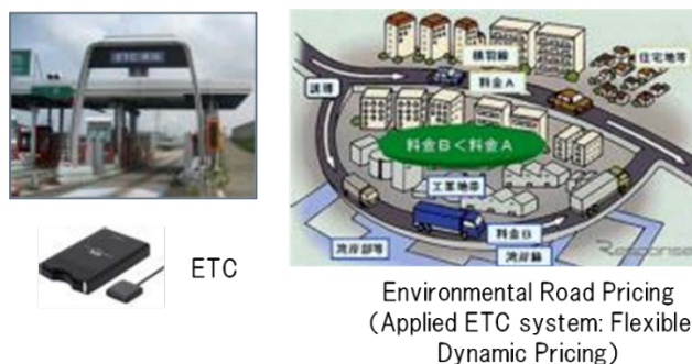
Source: Edited by JICA Study Team based on the materials of Metropolitan Expressway Co., Ltd. Figure 5-49 Electronic Toll Collection System
