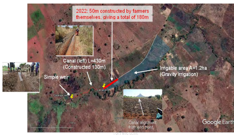
Figure 11 Photo and Location Map of a Simple Weir and Earthen Canals Constructed Through the Pilot Project (Calange Site)
