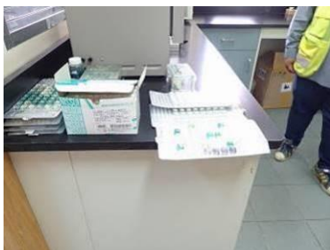
Simplified fecal coliform analysis (Water quality laboratory in sewage treatment plant in Buraydah city)
