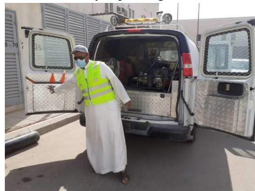
Helium gas survey vehicle with helium gas generator
