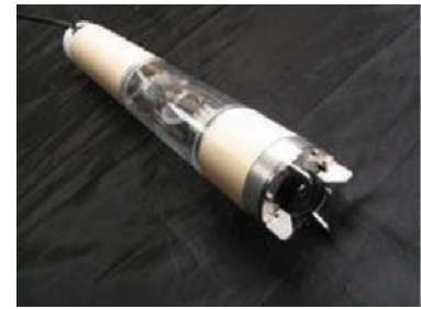
In-pipe survey robot
