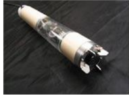
Photo 4-22: In-pipe investigation robot
