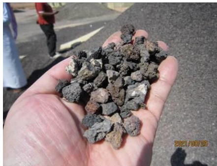
Photo 4-11: Natural water retention material
