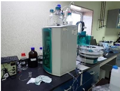
Bromine analysis using ion chromatograph
