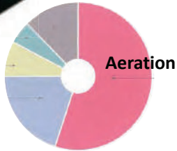
Power Consumption in WWTP
