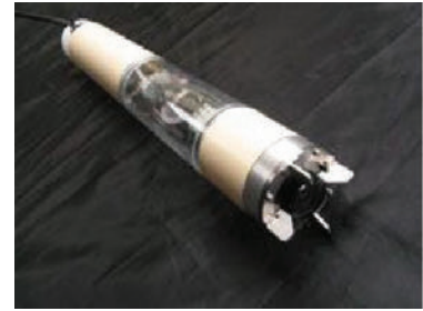
In-pipe survey robot
