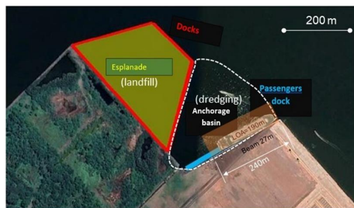
Figure 5-11 Location of Ro-Ro berth on Option-1 and a landfill for the disposal site
