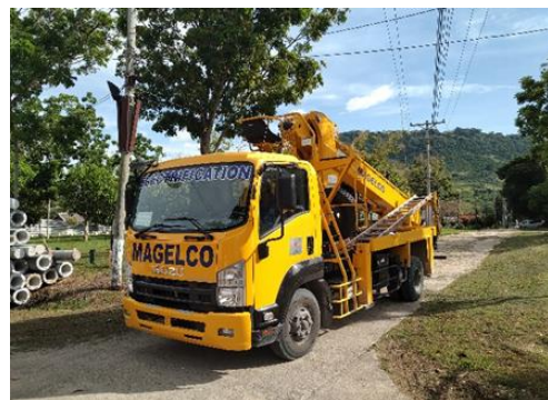
(b) Boom Trucks with Digger
